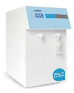
With LCD controlling system, 2 way water quality sensor, timing and quality dispensing, single stage RO system,1 pump, and built-in 12 liters tank, *Eco-Q* series *deionized water system* is *economic choice* of deionized water for general grade experiments.
