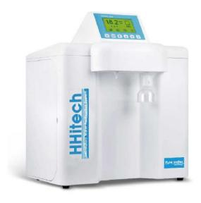
With LCD controlling system, 3 way water quality sensor, timing and quality dispensing, single stage RO system and 2 pumps, *Master-S* series *ultrapure water system* is *superior choice* of ultrapure water for high grade experiments.
